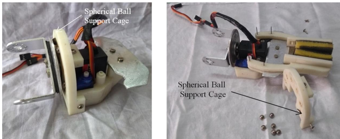
Figure 2.5.1 Spherical balls support cage (Assembled and Disassembled)
