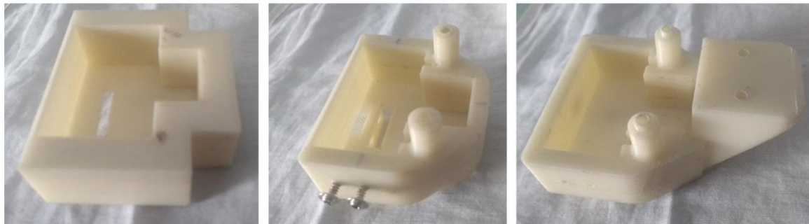
Figure 2.1.1.1 Evolution of the gripper body (from left to right)
